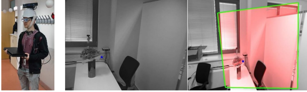
Figure 3. Experimental setup of the second series of experiments (left), Visualization of a homography: eye-tracker image (middle), Kinect image (right). Blue dot is the measured gaze position.
