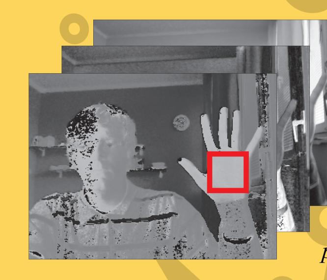
• The color filter segments an image according to ranges of saturation and value (lightness).
